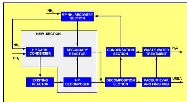
Fig. 9 - Conventional Total Recycle plant revamped with the HEC concept
