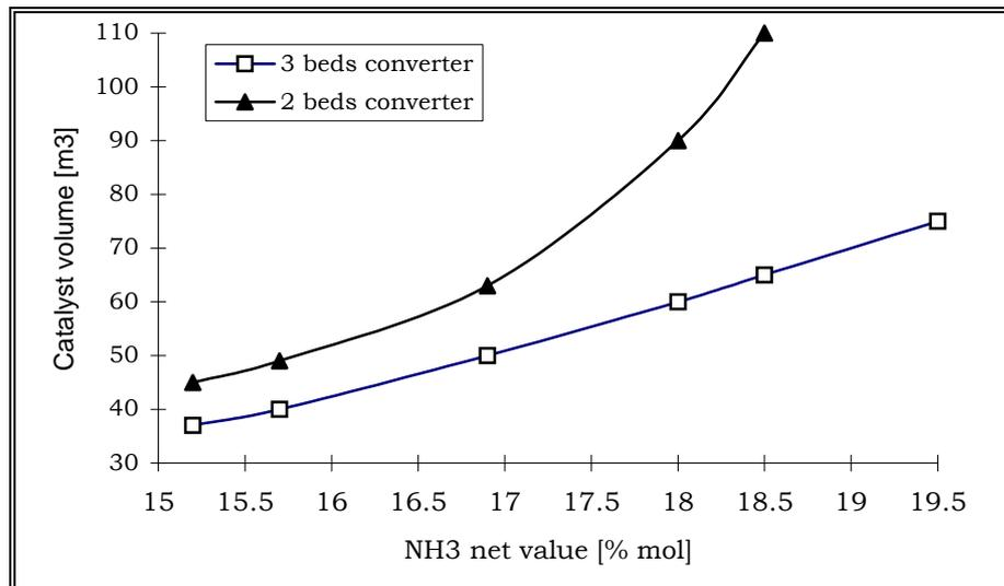
Fig. 7 - Catalyst volume versus NH<sub>3</sub> net value
