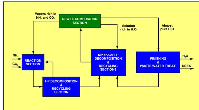
Fig. 10 - Stripping plant revamped with the VRS concept
