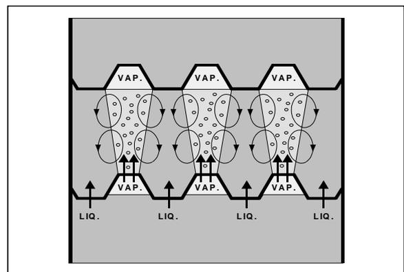
Fig. 8 - High Efficiency Reactor Trays
