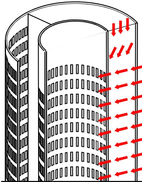
This feature is an essential factor for an easy and simple construction of any type of converter internal and for an effective elimination of the catalyst caking problem.
