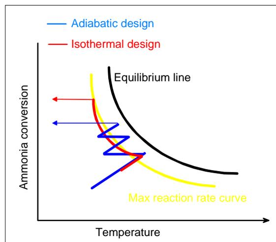
**Fig. 4 - Temperature Profile of the IAC**
