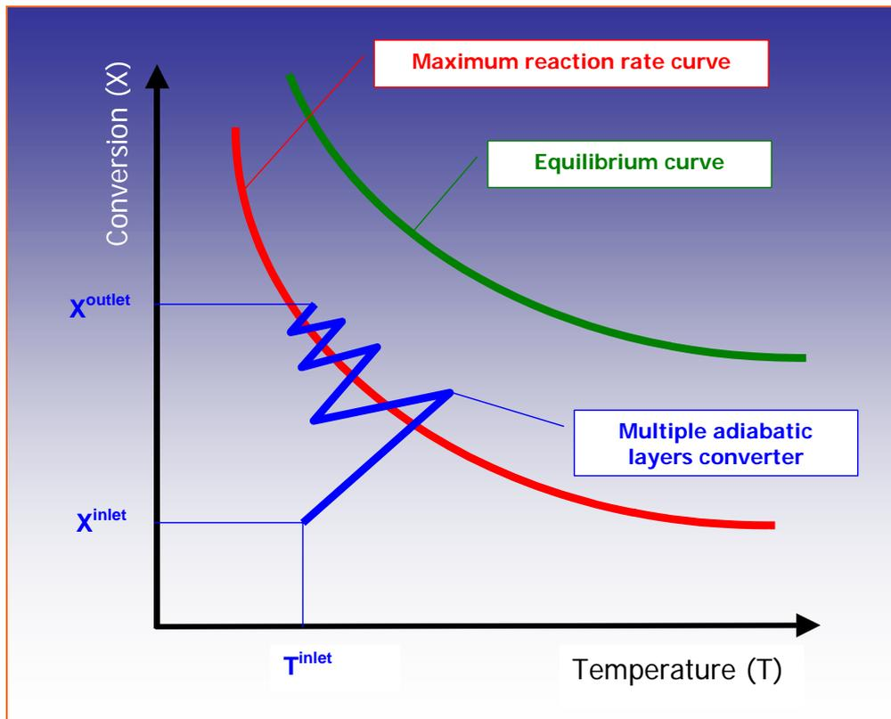
**Figure 2** – Path followed by multiple adiabatic layers converter in Conversion-Temperature graph.
