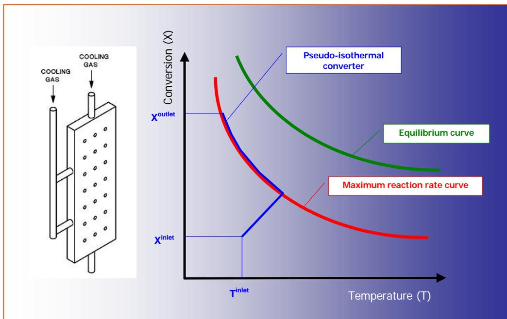
**Figure 4** – Injections of coolant fluid in plate cooling device and converter behaviour.
