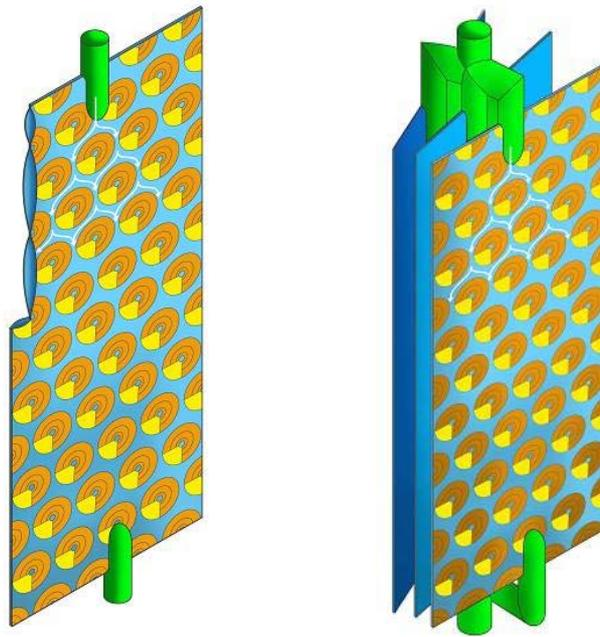
**Figure 3** – Sketch of a single element and of a bundle of plates.
