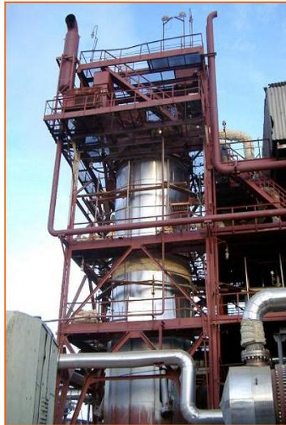
**Figure 9** – *The first plate-cooled methanol converter.*
