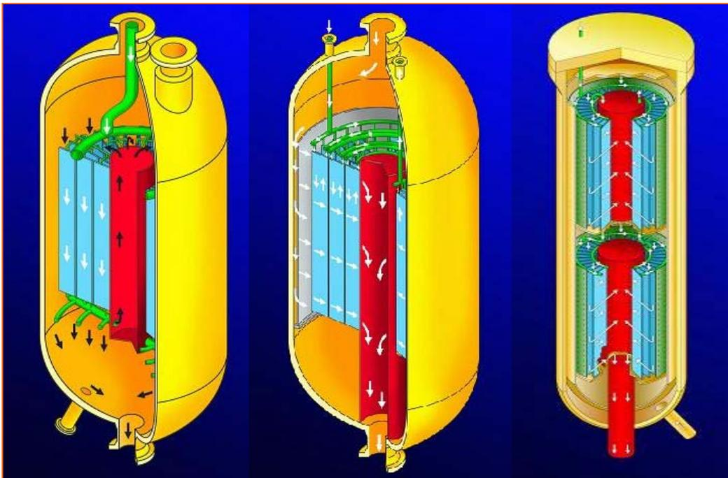
**Figure 5** – *Examples of pure axial and axial-radial plate-cooled single converter and multiple-bed converters, e.g., a typical arrangement used in an ammonia converter.*
