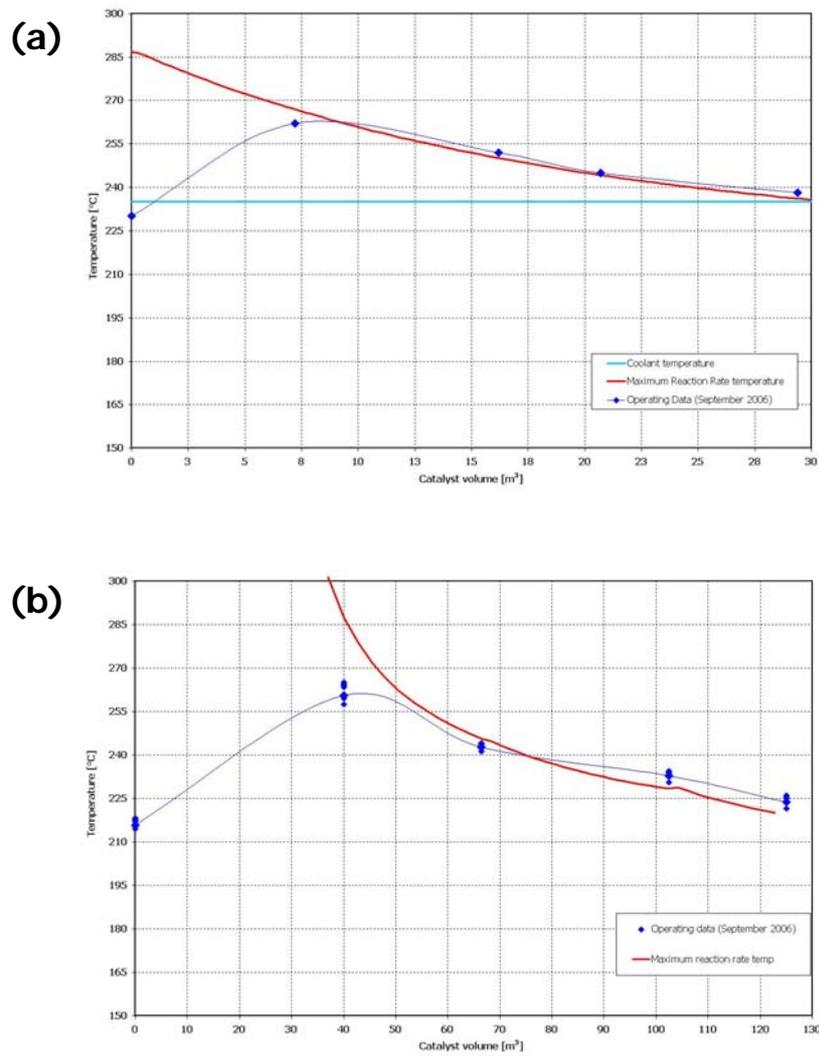
Figure 11 – Example of methanol converter operating conditions.
