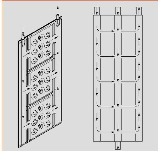
**Figure 6** – *Example of plate arrangements for axial-radial beds.*
