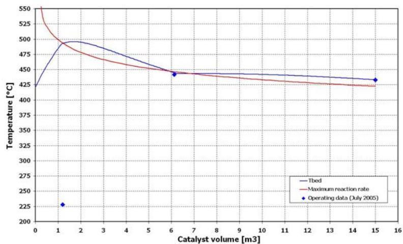
Figure 12 – Example of ammonia converter operating conditions.
