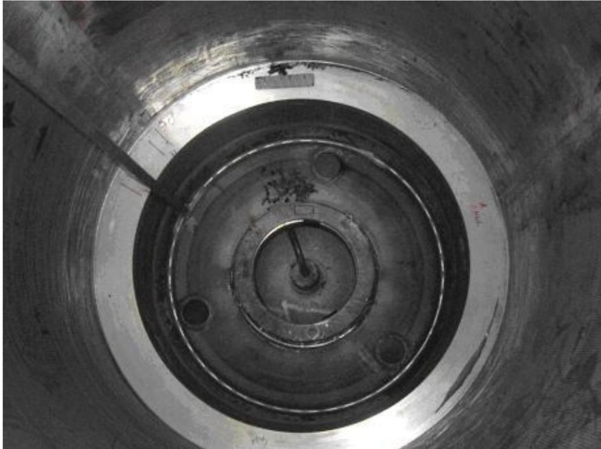
To feed the synthesis gas into the central part of the converter (inlet distributor), Casale designed a cover diverting the gas to the bottom and the support point of the cartridge with a free zone to allow the gas to flow through. This feature results in high reliability of the design because it eliminates the need for an expansion joint by eliminating the need for a central pipe to feed the gas to the catalyst bed. Expansion joints have the possibility of failure.
