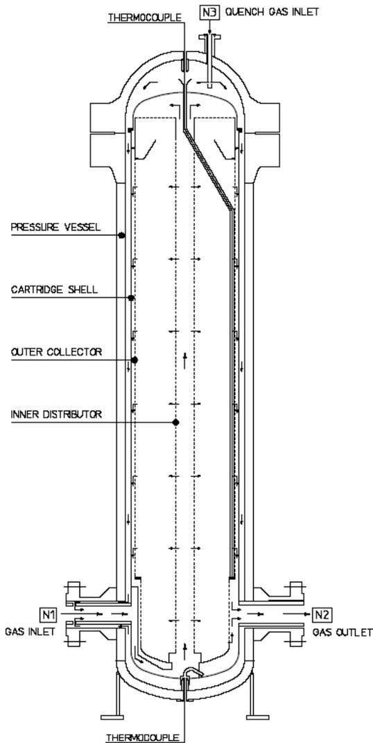
After leaving the catalytic bed, the gas flows through the outer collector to the bottom part of the cartridge and exits the converter through nozzle N2.
