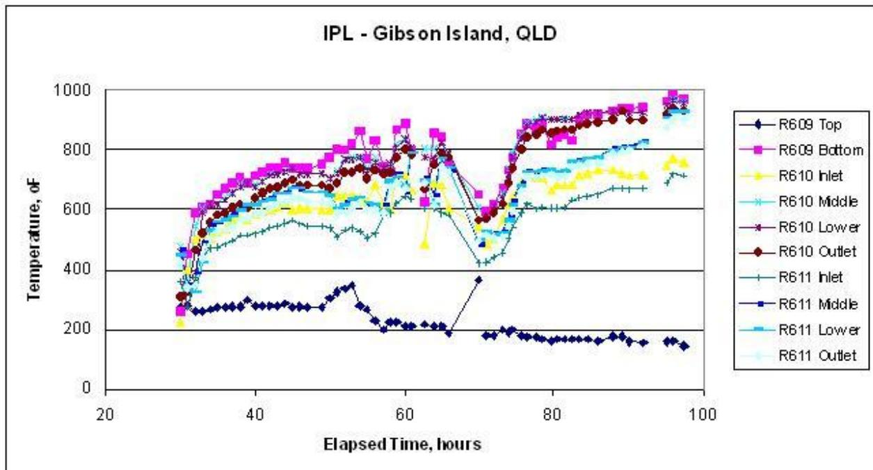
As can be seen from these graphs, the total reduction time was approximately 4 days. However, the first day was not productive since troubles with the Startup Heater (SUH) resulted in most of the day lost. So, assuming no compressor or SUH problems, reduction could have been completed in 3 days. It must be pointed out that water evolution during the reduction was faster than targeted due to the large SUH in the loop.
