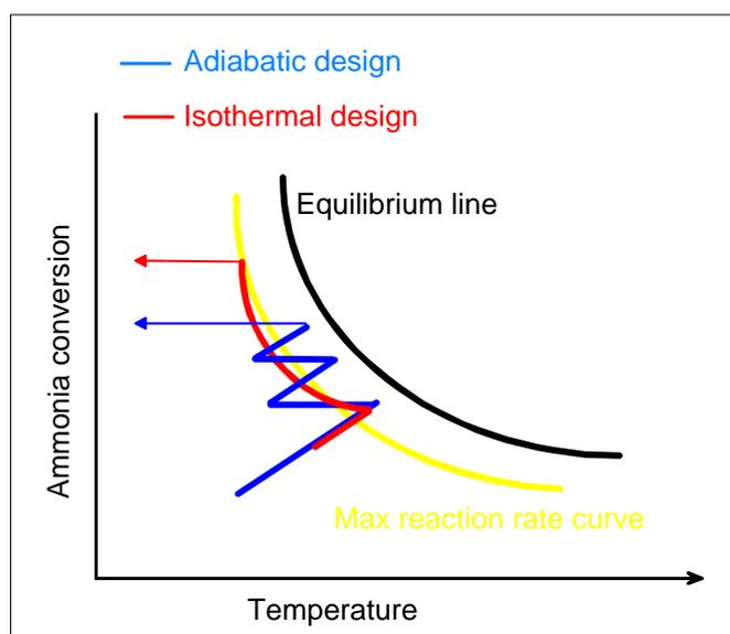
**Fig. 7 - Temperature Profile of the IAC.**
