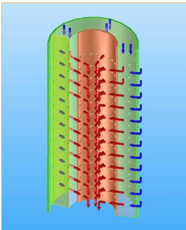
**Fig. 1: Gas Distribution in an Axial-Radial Catalyst Bed**
