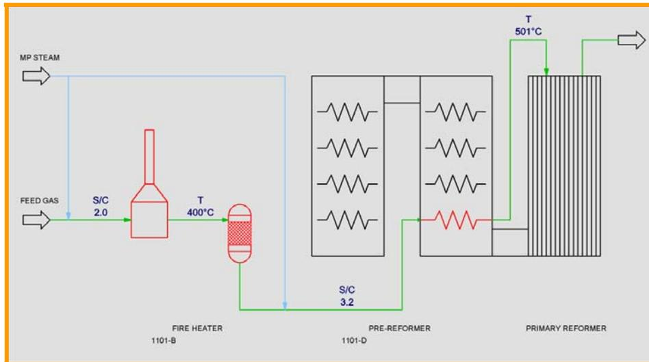
**Fig. 3: New Fired Heater and Pre-Reformer**
