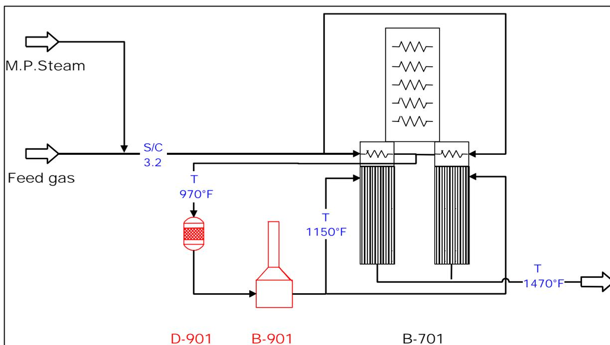
**Fig. 5 - Pre-Reformer Arrangement, new items in red.**
