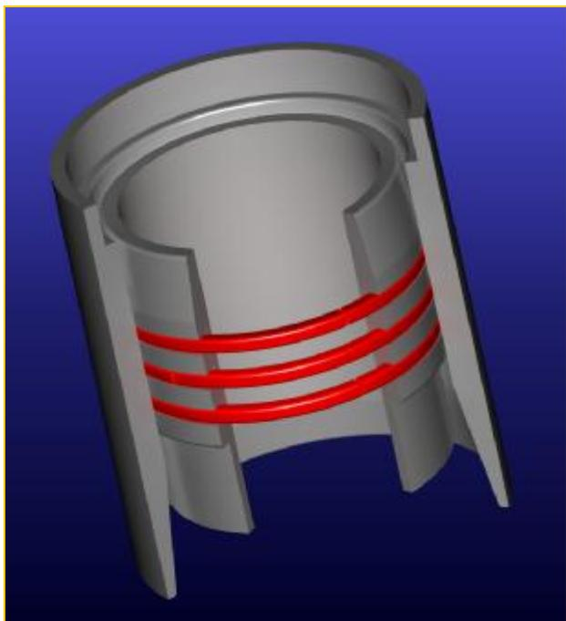
**Fig. 7 - Elastic Ring Seal**
