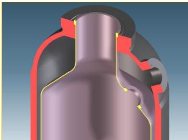
**Fig. 5 - Manholes in Partial Opening Converters**
