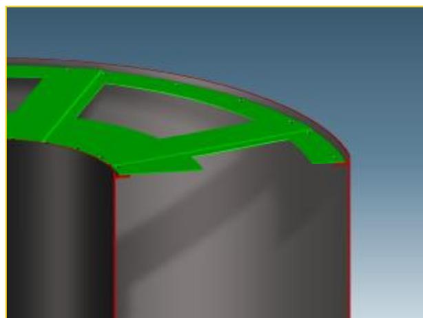
**Fig. 6 - Axial Radial Flow Protection Screens**
