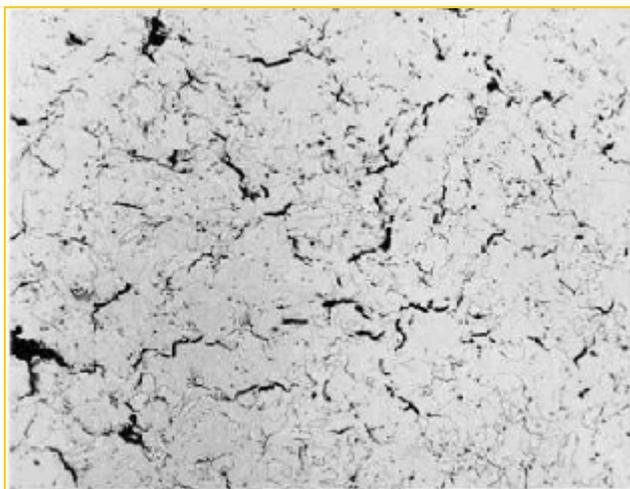
**Fig. 1 - High Temperature Hydrogen Attack**
