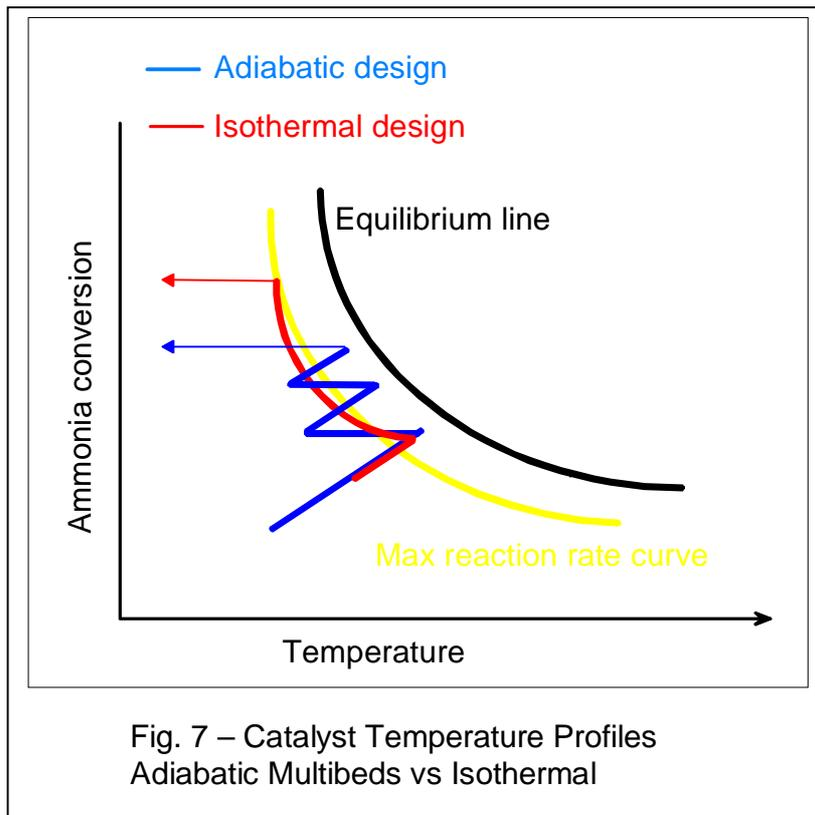
The construction of pseudo-isothermal converters is nothing new, as it was practiced since the early years of the ammonia industry by Casale and others. In the old design efficiency and maximum capacity was limited though, because the catalyst bed was axial and the cooling elements were tubes fixed to a tube-sheet.
