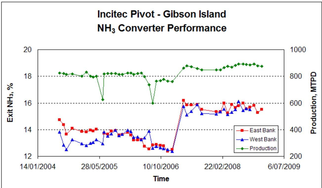
It is possible to see that after the revamping in March 2007 the production rate and the conversion per pass has increased sharply.
