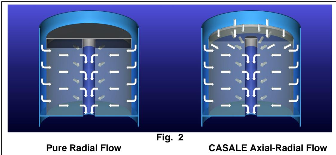
There is a protection screen installed on the top of the catalytic bed allowing gas to flow axially through the top part of the bed.
