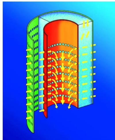
Figure 2. Axial-radial design for catalytic beds
