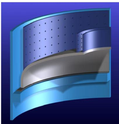
Figure 3. Casale catalytic bed bottom
