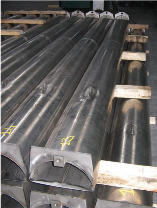
**Fig. 4 – Tubular collectors**
