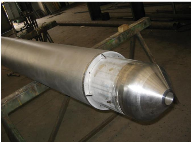
Fig. 13 – CASALE ATR burner installed in a two-step reforming 1,350-MTD methanol plant before installation in May 2004
