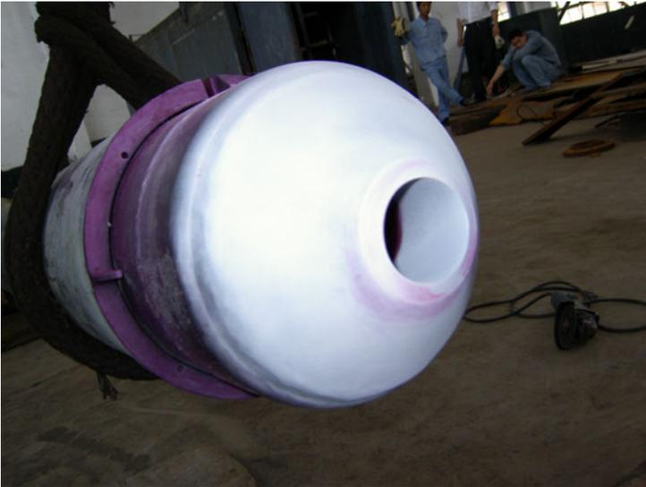
**Fig. 14** – Same burner as in Fig 13 during a periodic turnaround. The liquid penetrant test shows no evidence of cracks or damage due to thermal fatigue
