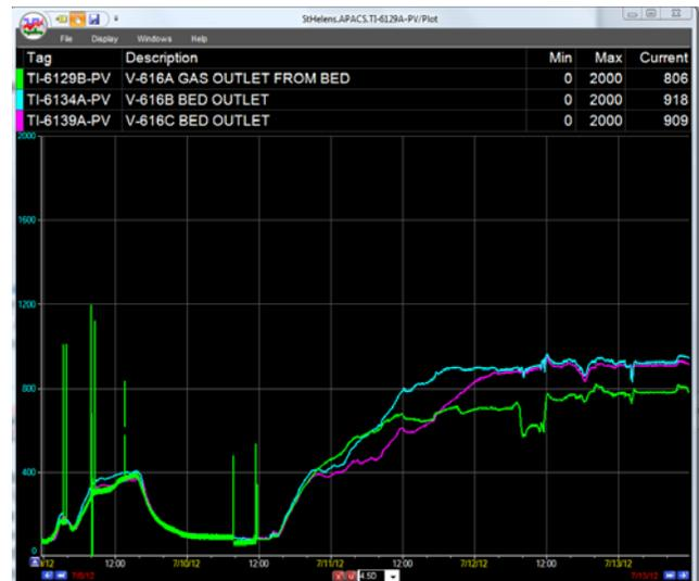
Figure 13. Catalyst reduction chart – V-616A, B, C reduction temperatures vs time
