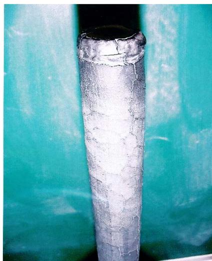
Figure 2. Cracked Thermowell Guide (2001)
