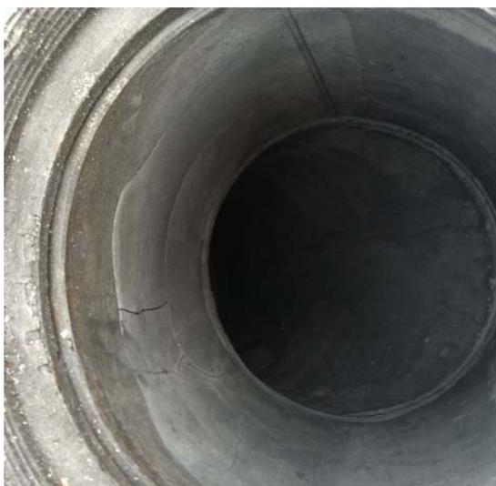
Figure 3. Cracking seen in V-616A outlet nozzle
