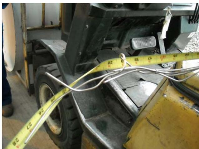
Figure 14. Thermocouple bundle that was bent going in
