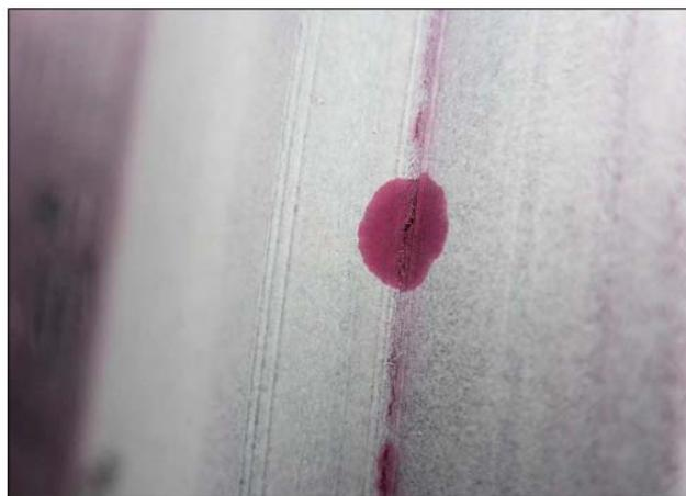
Figure 5. Cracks noted in ring joint gasket groove of the top head of V-616A
