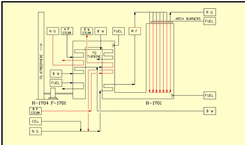
Fig. 2: Retrofitted Reformer Process Scheme
