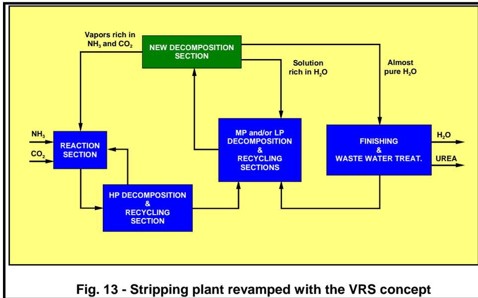
Fig. 13 - Stripping plant revamped with the VRS concept
