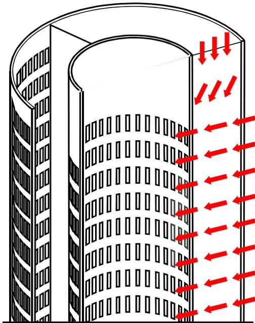
**Fig. 9 - Axial-radial Bed,
