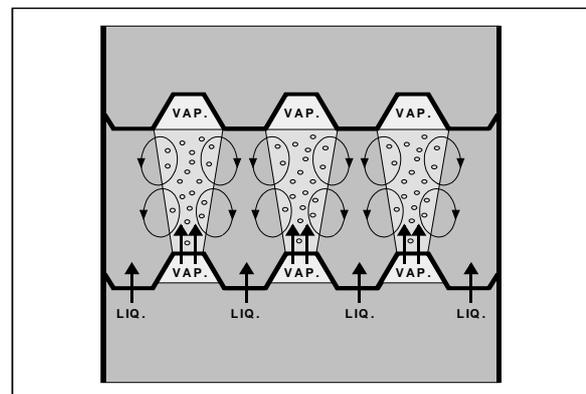
**Fig. 11 - High Efficiency Reactor Trays**
