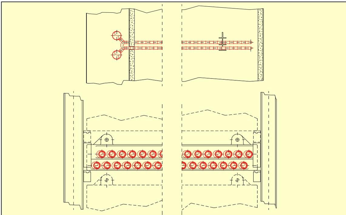
**Fig. 5: New Natural Gas Preheater**
