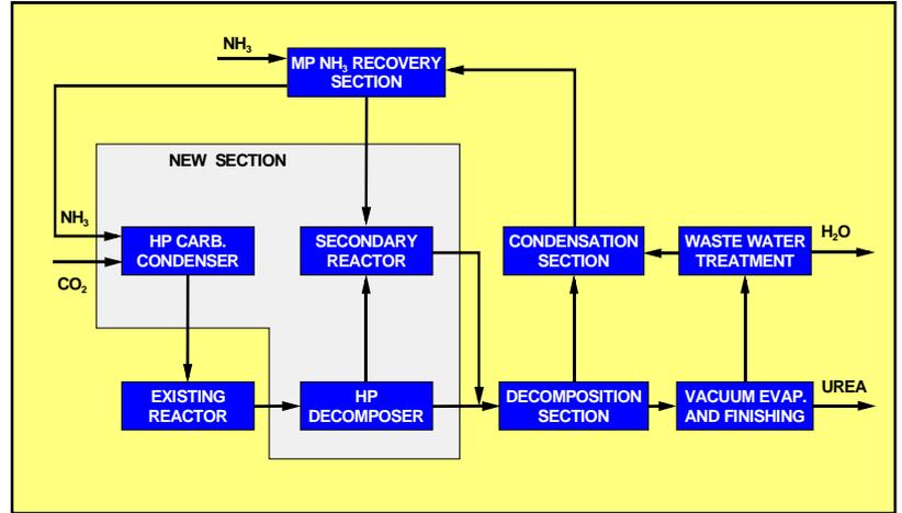
Fig. 12 - Conventional Total Recycle plant revamped with the HEC concept
