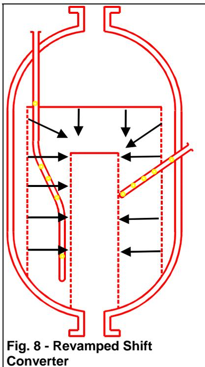
This new configuration has an inherently low pressure drop of the catalyst bed, and in addition, makes it possible to use small-size, more active catalyst.
