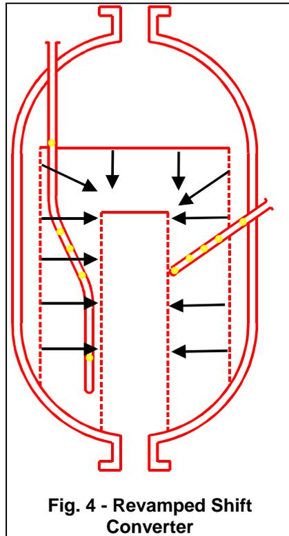
The new axial-radial configuration has an inherently low pressure drop of the catalyst bed, and this makes it possible to use small-size, more active catalyst.
