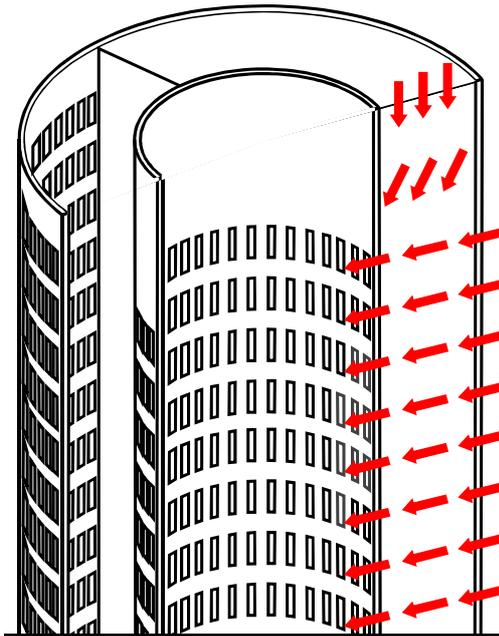
Fig. 1 - Axial-radial Bed,
