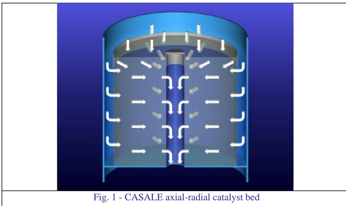
In the axial-radial concept, the distribution of the gas is achieved by the perforated walls, which ensures a low pressure drop, stable with time as the catalyst ages or deteriorates, irrelevant also to caking of the catalyst top layer due to water droplets carry-over. Hence, by ensuring a higher suction pressure to the compressor through the catalyst life, it achieves a higher production rate.
