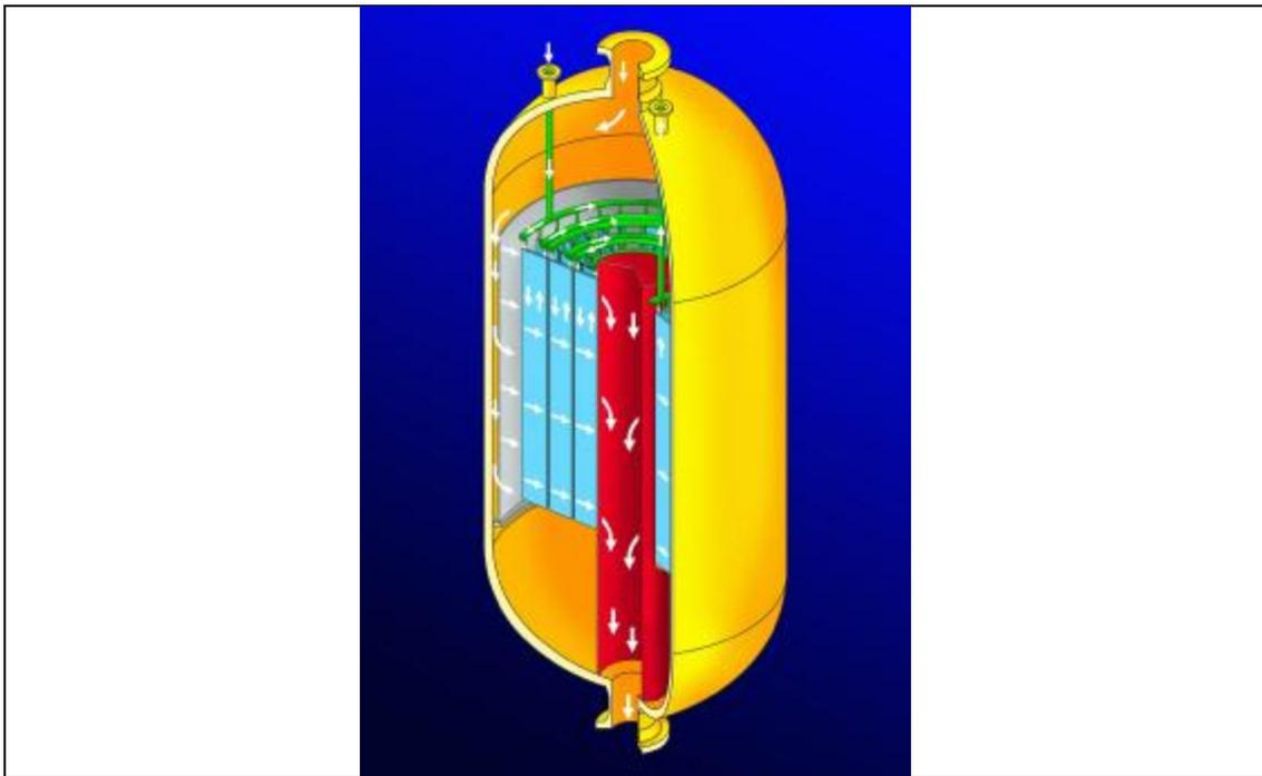
Figure 5 - CASALE Isothermal Methanol Converter
