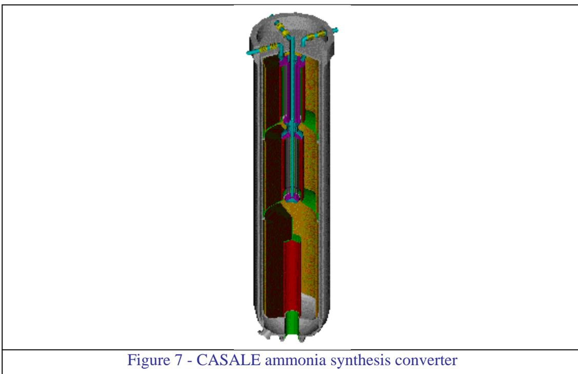
The three catalytic beds have axial-radial flow, to minimize the nozzle-to-nozzle pressure drop.
