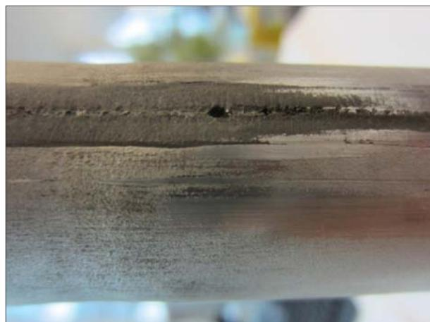
*Fig. 5. Typical localized corrosion of a welded tube*
