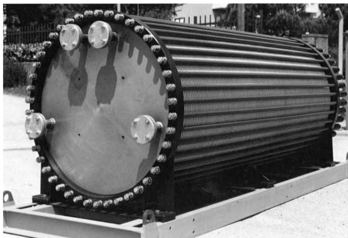
*VOLTIANA® cell stack producing 100 Nm<sup>3</sup>/h hydrogen at 10 bar pressure*
