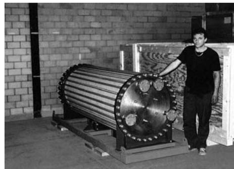
*Three views of VOLTIANA cell stacks, respectively for 500, 5 and 350 kW rated power (approx 120, 1.2, 80 Nm<sup>3</sup>/h hydrogen production)*
