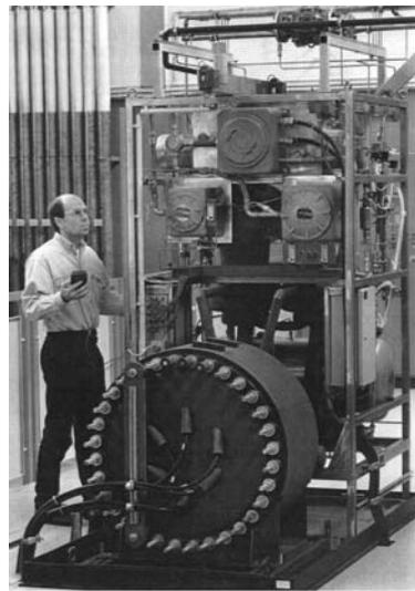
*VOLTIANA<sup>®</sup> electrolysers producing, respectively, 2 Nm<sup>3</sup>/h hydrogen at 30 bar, and 7 Nm<sup>3</sup>/h hydrogen at 6 bar under PV power*
