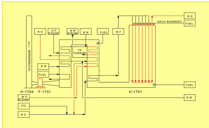
**Fig. 3 – New Reformer Process Scheme**
