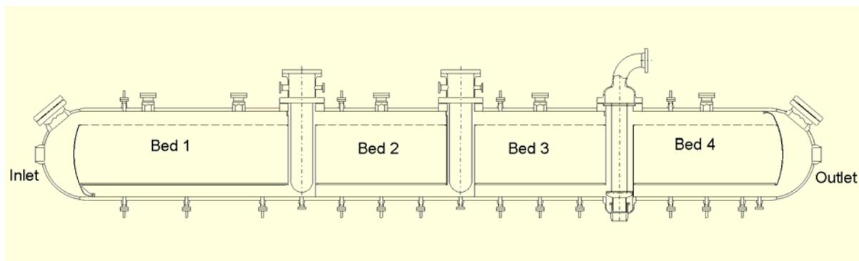
**Fig. 4 – Horizontal Converter**
