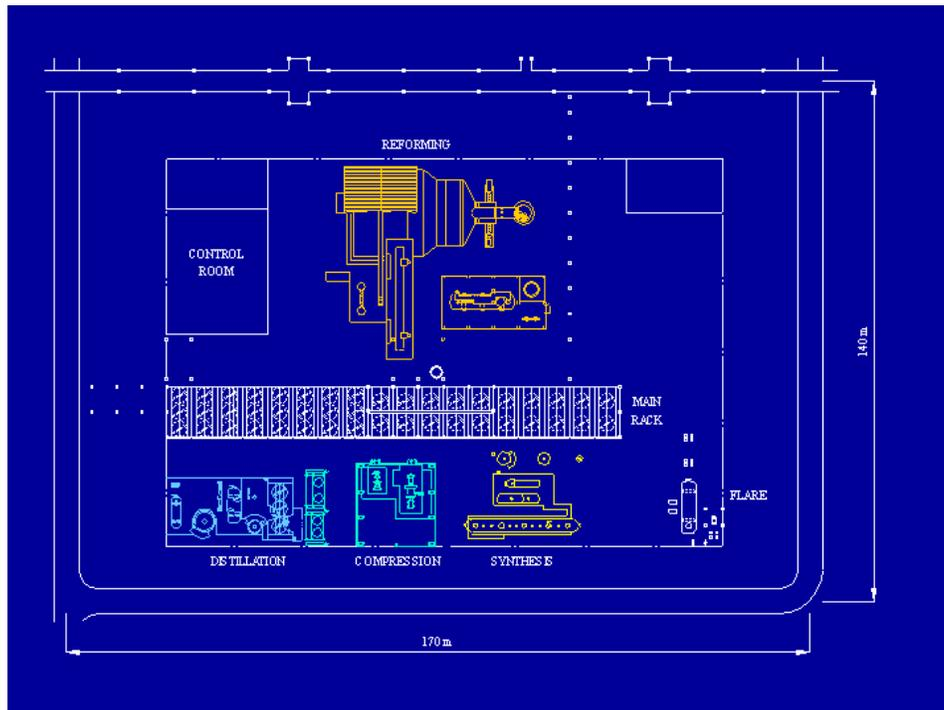
**Fig. 7 – Simplified Plant Layout of New Methanol Plant**
