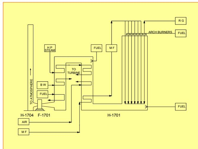
**Fig. 2 – Existing Reformer Process Scheme**
