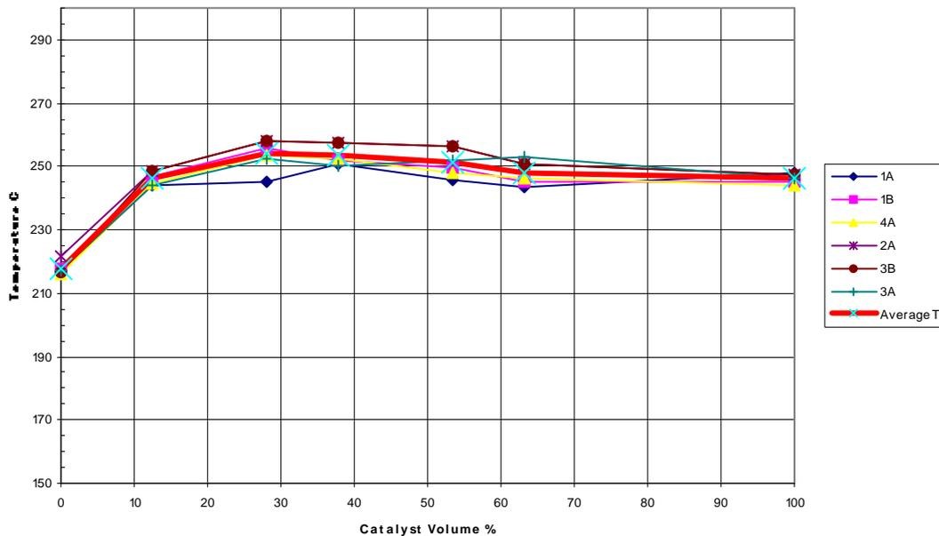
As it can be seen the temperature profile is very smooth, with very little dispersion of the temperature value around the average.
