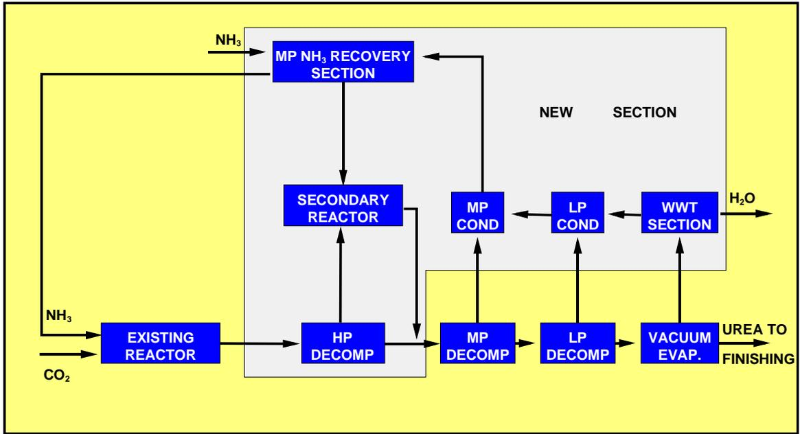
Fig. 3 – Partial Recycle Plant revamped with HEC concept
