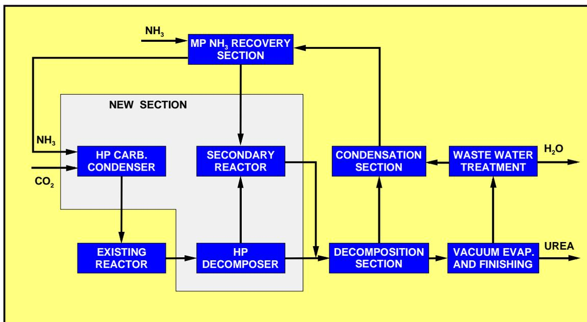
**Fig. 2 - Conventional Total Recycle plant revamped with the HEC concept**
