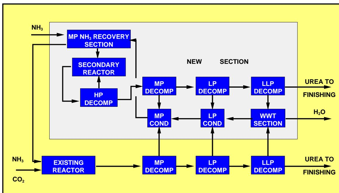
**Fig. 5 – Simplot Canada Ltd. Plant revamped according to HEC concept – Block Diagram**
