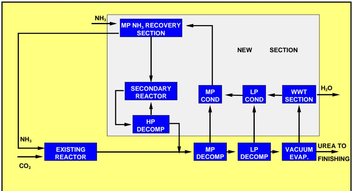
Fig. 4 – Partial Recycle Plant revamped with HEC Concept
