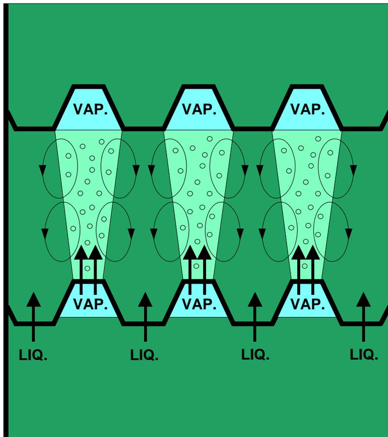
Fig.4 - Casale-Dente High Efficiency trays
