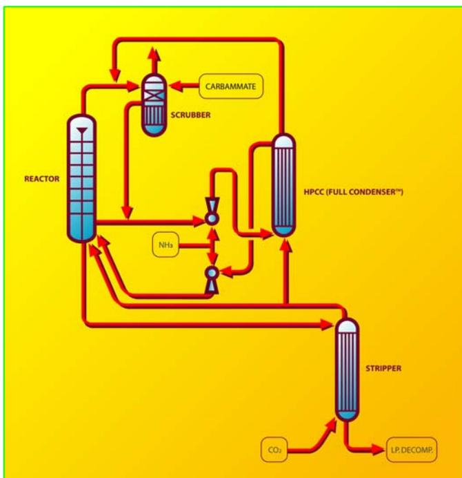
**Fig. 10 - Split Flow Loop™ configuration**
