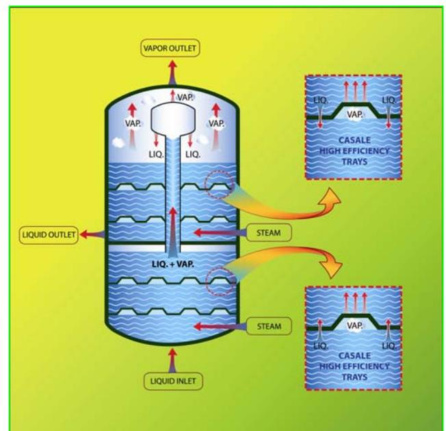
**Fig. 2 - High Efficiency Hydrolyser**
