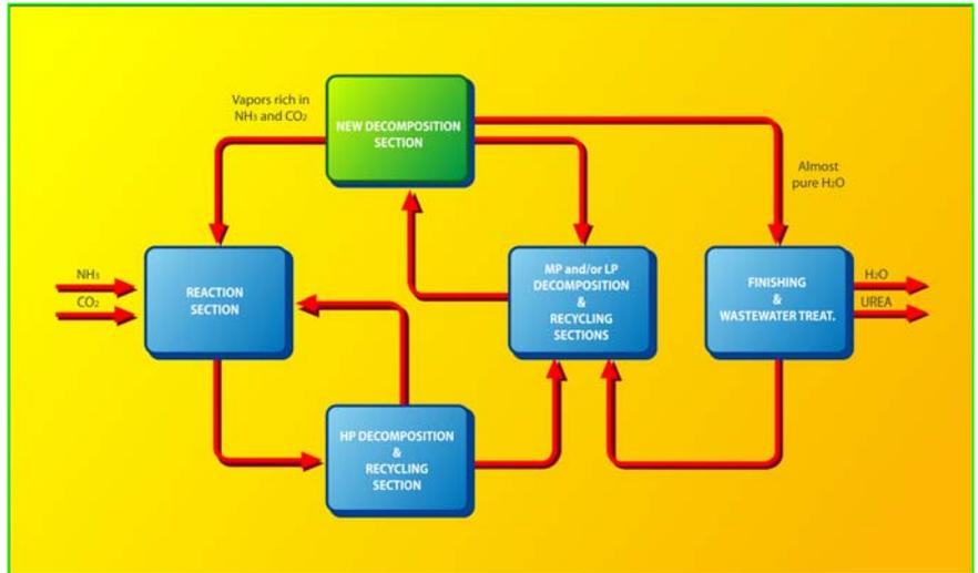
**Fig. 4 - Stripping Plant Revamped according the VRS Concept**
