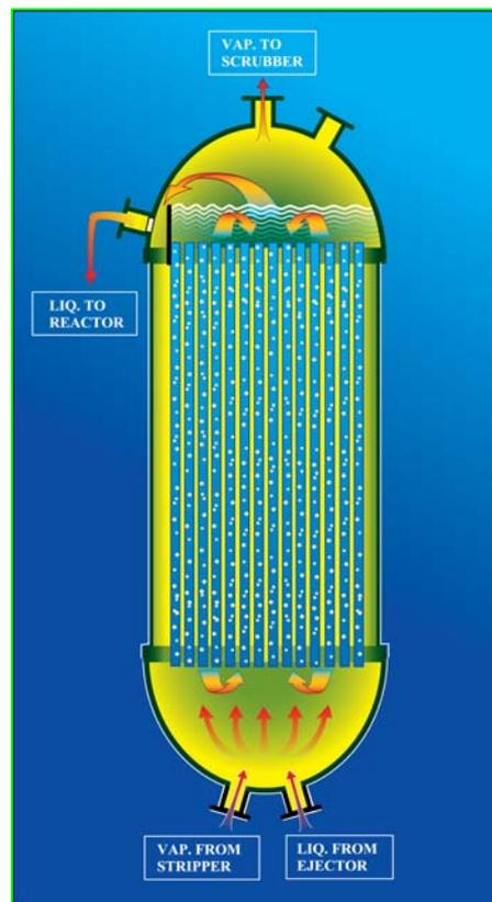
**Fig. 9 - Full Condenser™ configuration**
