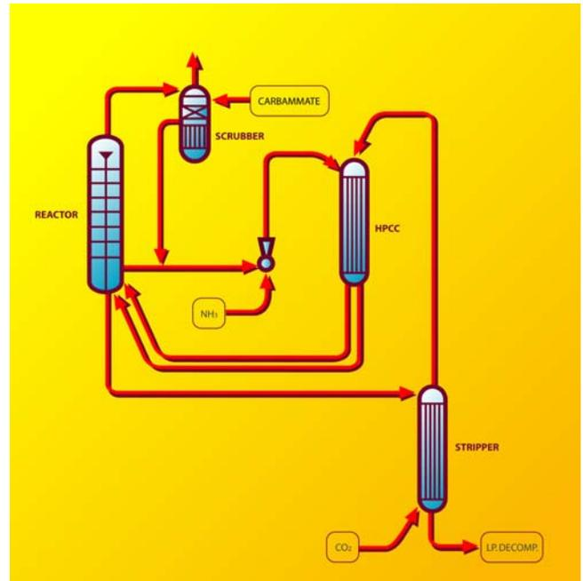
**Fig. 5 - HP Loop of CO<sub>2</sub> Stripping Plants**
