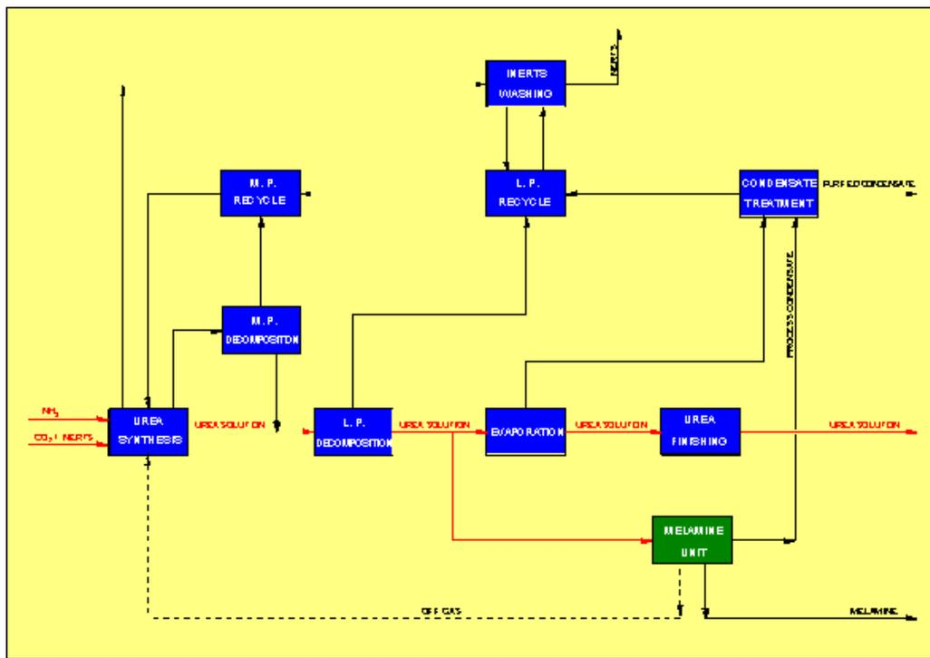
FIG. 9: UREA CO<sub>2</sub> STRIPPING PROCESS INTEGRATED WITH AGROLINZ MELAMINE PROCESS
