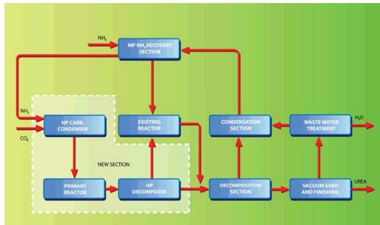
FIG. 3: CONVENTIONAL TOTAL RECYCLE PLANT REVAMPED WITH THE HEC CONCEPT
