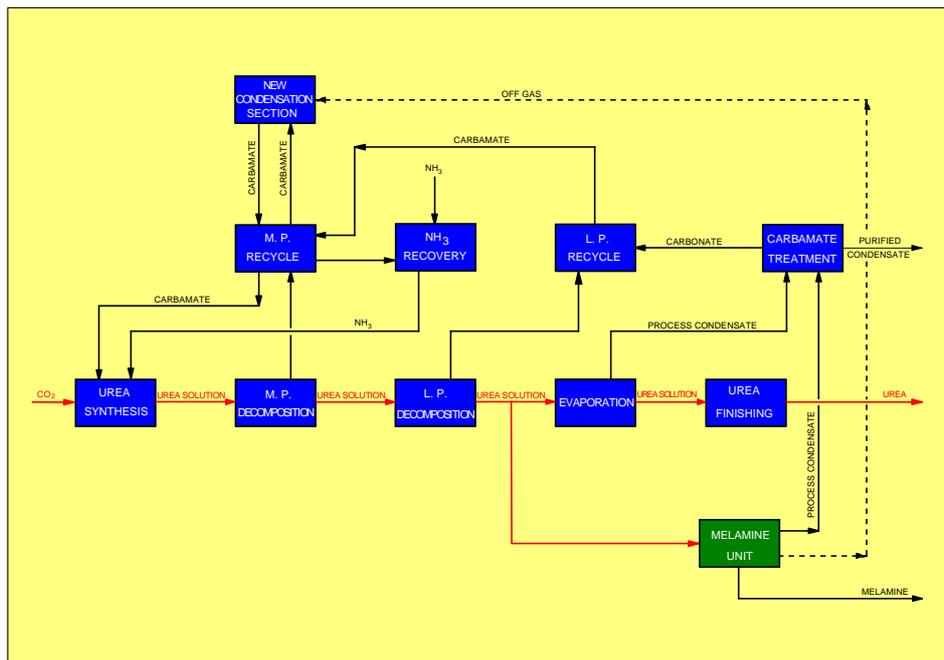
FIG. 11: UREA TOTAL RECYCLE PLANT INTEGRATED WITH EUROTECNICA MELAMINE PROCESS
