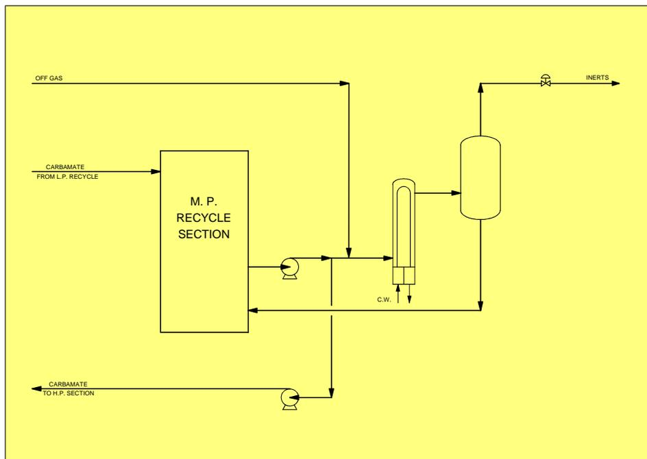
FIG. 13: NEW OFF-GAS CONDENSATION SECTION
