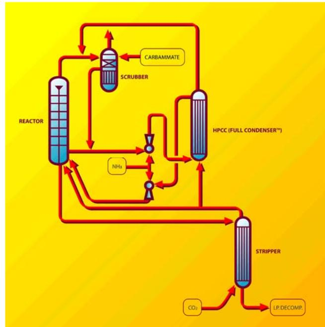
FIG. 5: SPLIT FLOW LOOP™ CONFIGURATION
