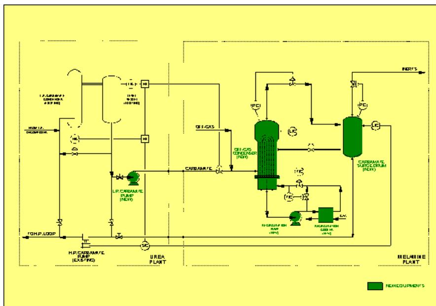
FIG. 8: NEW OFF-GAS CONDENSATION SECTION
