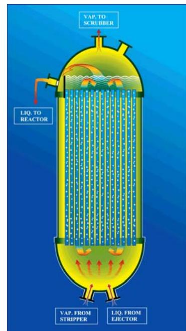
FIG. 4: FULL CONDENSER™ CONFIGURATION
