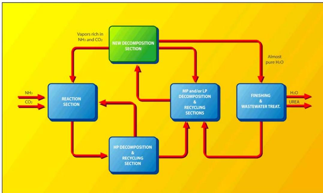
FIG. 6 - STRIPPING PLANT REVAMPED ACCORDING THE VRS CONCEPT
