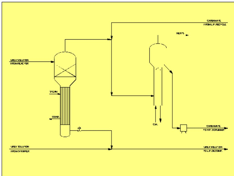
FIG. 10: NEW 20-BAR PARALLEL SECTION
