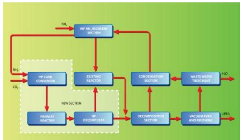
**Fig. 3 - Conventional Total Recycle Plant revamped with the HEC Concept**
