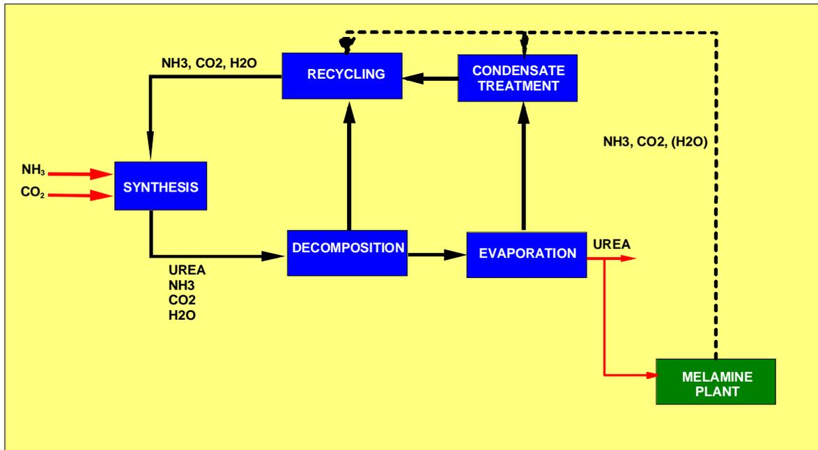
**Fig. 1 - Melamine Plant Integrated with Urea Plant**
