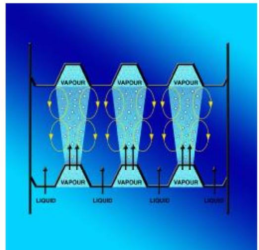
**Fig. 2 - Casale-Dente High Efficiency trays**
