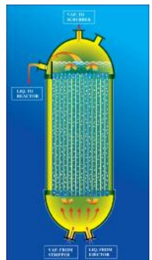
**Fig. 4 - Full Condenser configuration**
