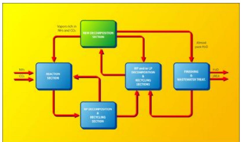
**Fig. 6 - Stripping Plant Revamped according the VRS Concept**
