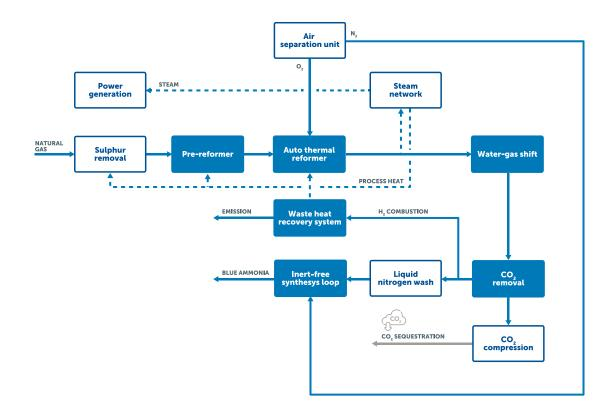
**Ammonia Synthesis** - After adding with  $N_{2'}$ , the purified, inert-free syngas is compressed and directed to a Casale ammonia synthesis loop, equipped with a Casale Axial-Radial<sup>®</sup> ammonia converter, where low-carbon, cold ammonia is produced. The high efficiency of the converter and the reactivity of the inert-free gas ensure that equipment sizes in the synthesis loop and refrigeration section are within the limit of industrially proven references.
